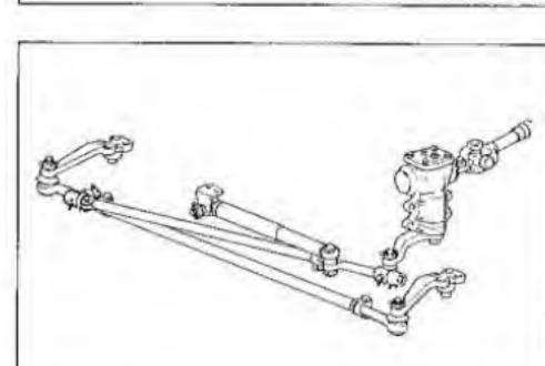
INSPECT STEERING LINKAGE, GEAR BOX, STEERING WHEEL FREEPLAY, BALL JOINTS AND DUST COVER
